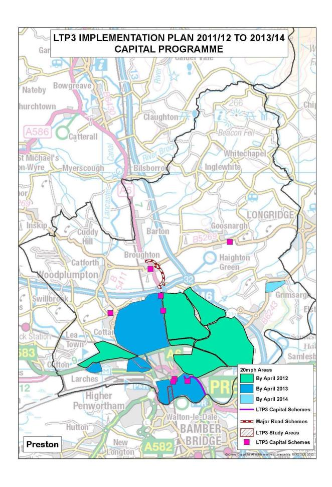
There will also be other minor improvements to the highway infrastructure to serve the developments at Whittingham and Cottam (PR3) and to the signalling along the A6 North corridor between the M55 and the city centre (PR4) to reduce delay and congestion.
